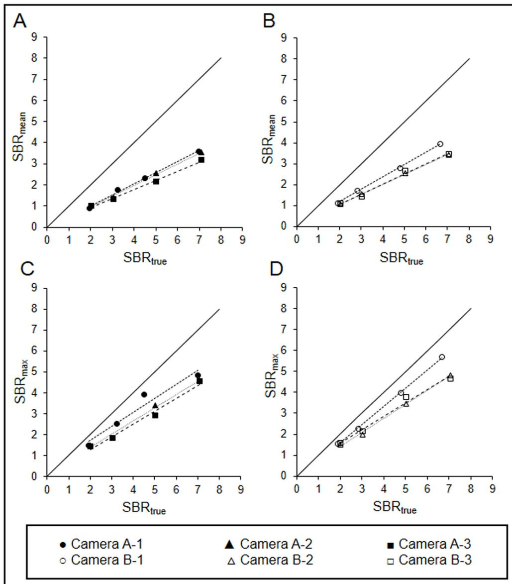
**Figure 3.** Correlation between  $SBR_{true}$  and  $SBR_{SPECT}$  of  $SBR_{mean}$  (A, B) and  $SBR_{max}$  (C, D), (A, C) Symbia T6, (B, D) Infinia Hawkeye 4 (Good linearity was observed for all collimators.)
