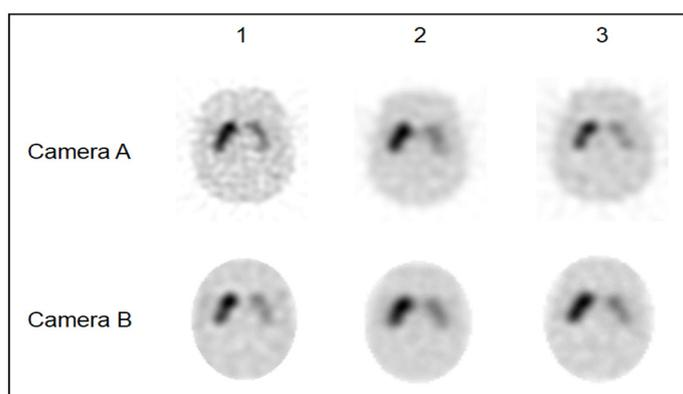
**Figure 2.** SPECT images reconstructed using the optimal reconstruction parameters (The images in the upper row were obtained using camera A, and the images in the lower row were achieved using camera B. The striatum was clearly observed on images using cameras A-1 and B-1.)
