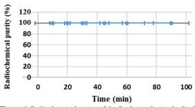
Figure 4. Radiochemical purity of the final complex in the final solution over 90 min
