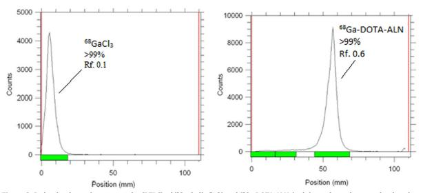
**Figure 3.** Radio thin-layer chromatography (RTLC) of  ${}^{68}$ Ga-GaCl<sub>3</sub> (left) and  ${}^{69}$ Ga-DOTA-ALN (right) on silica gel papers developed in 10% ammonium acetate:methanol (1:1) mixture as the mobile phase under optimized conditions
